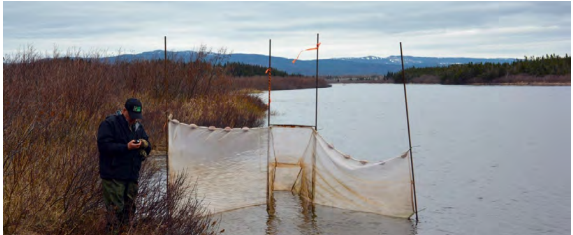
An Aboriginal River Guardian assisting QNR staff in the deployment of a fyke net. These nets are used to study the upstream migration of young eels as they first enter their home rivers.
