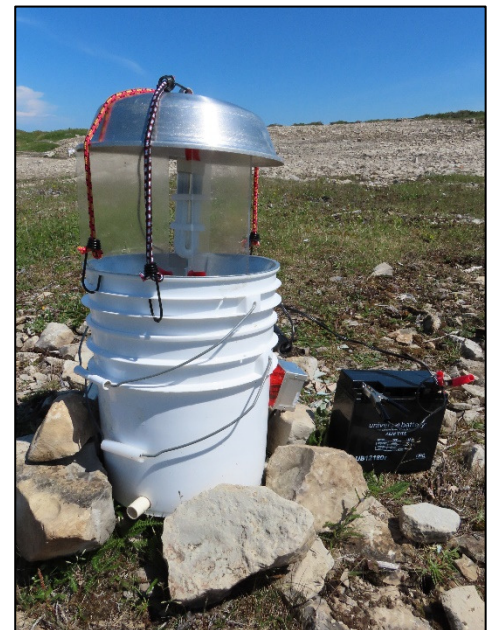
A light trap used to collect insect pests such as Diamondback Moth.
